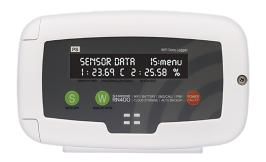
RN400-H2PS is designed to measure internal Temp/RH, and external NTC Temperature sensor signal and transfer them to the destination via WiFi connection. The destination would be an information system such as public cloud, local server, and even PC. It operates with battery power and has a protective gasket for various industrial sites. Premium RN400 H2 series have IP65 for protection, OLED screen for cold outdoor, F-RAM memory for instant backup and micro-SD card for CSV backup.
